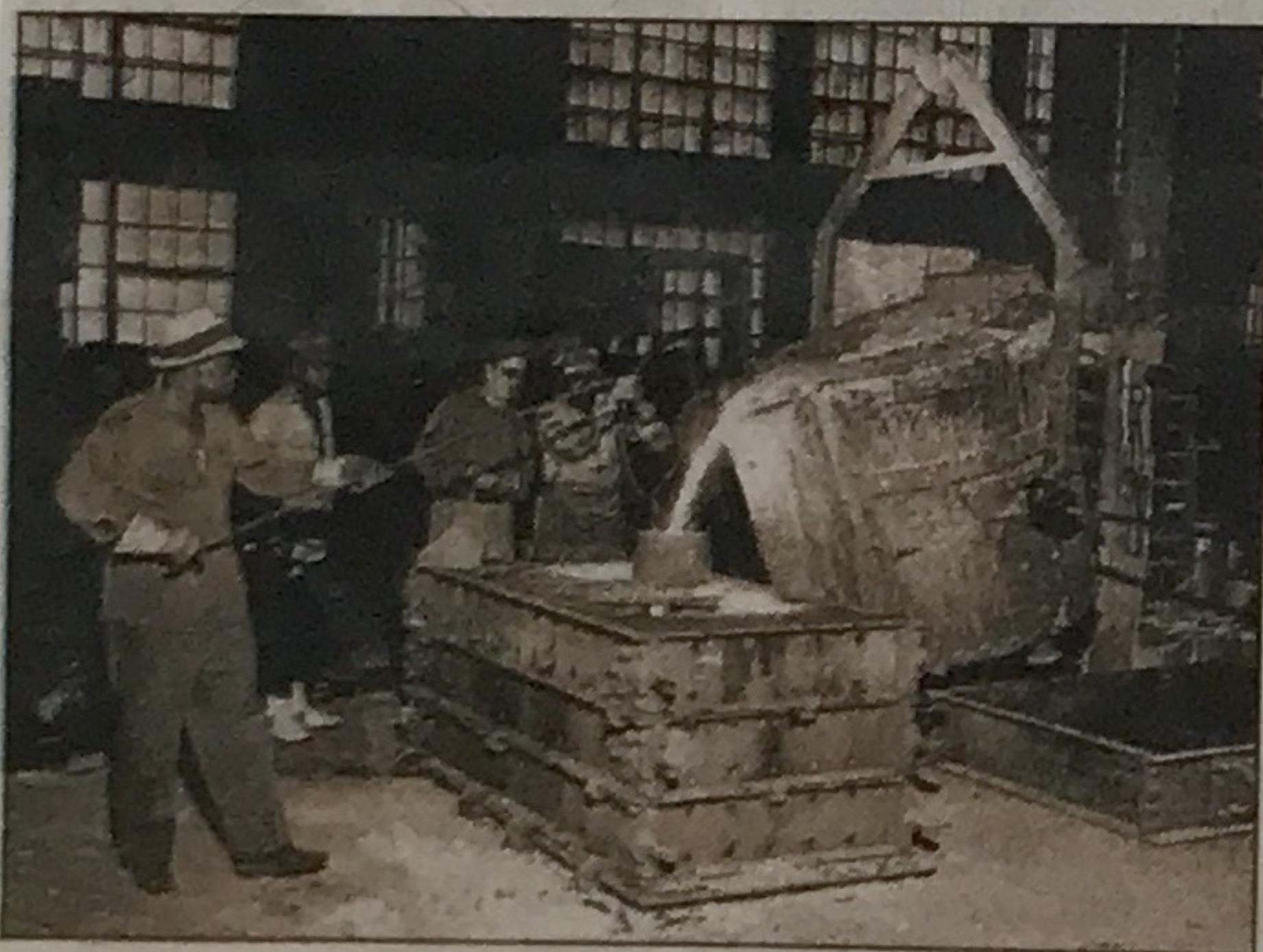
Employees pouring molten iron into a mold in the 1950s.
